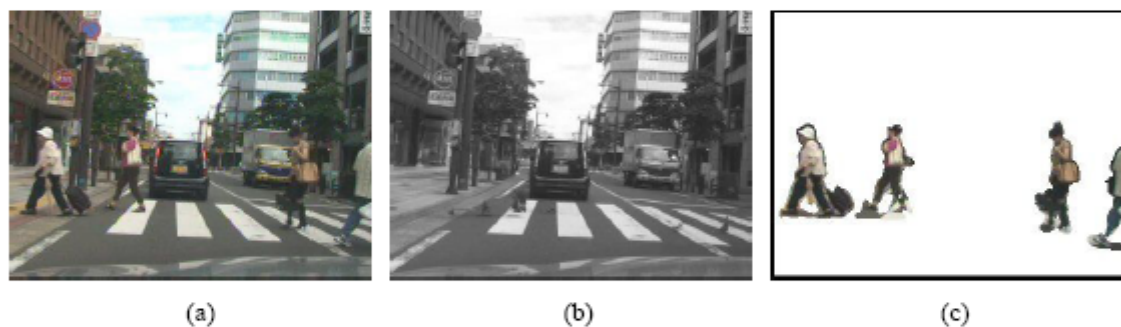
Fig. 4. Experimental result_2: Images from a video camera mounted on a car. (a) Original video images; (b) the obtained backgrounds; and (c) extracted moving objects.
